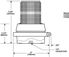
Standard mounting options are 1/2" (13mm) conduit, direct surface or 4" (102mm) octagonal box.
