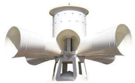
The EWS-V3 is available in single phase or three phase and is a single tone siren, producing 460 cycles per second, for optimal sound penetration. All exposed siren components are of metal construction, which are "powder coated" for a durable finish. The fan and housing are made of non-corrosive cast aluminum
