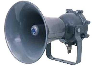
The 5533M and 5533MD signals are explosion-proof, heavy-duty industrial, tone-selectable, audible signaling devices capable of producing volume-controlled, high-decibel tones. The signal accepts up to two contact closures and delivers one or two audible output signals selected from the 55 tones available.
