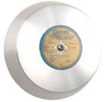
The Edwards 338 and 339 are surface mount AC or DC single stroke chimes which can be pulsed up to 10 pulses/second. The chimes are high quality units with underdome construction intended for heavy-duty commercial and industrial use. The chimes require no lubrication, and come complete with an Adataplate® mounting plate.
