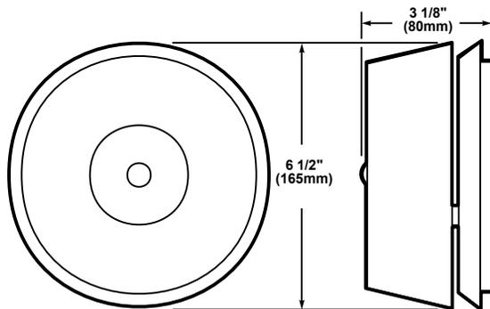
Mounts on any plaster cover with mounting holes on 2 3/4" (70mm) centers, on any single gang opening, on any 3 1/4" (83mm), 3 1/2" (89mm), or 4" (102mm) octagonal box or 4" square box. Also mounts directly on any wall surface.
