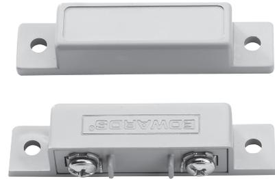
Edwards magnetic switches are designed to activate a variety of signaling devices. Normally open circuits close when the magnet engages. SPDT switches are for open circuit systems or for central office operation. Normally closed circuits open when the magnet engages. For accessories, see Magnetic Switch Accessories, page 10-24.
